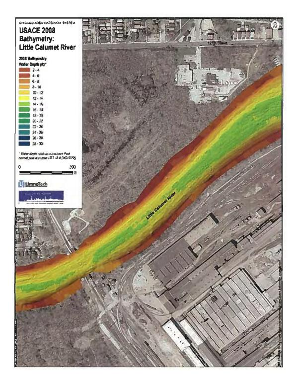
Figure 3-5: Example of CAWS Bathymetric Data in GIS.
