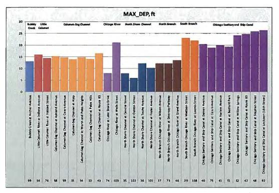
Figure 4-6: Maximum Channel Depth at CAWS Sampling Stations<sup>4</sup>.
